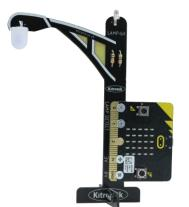
**Connection:** 4 x M3 countersunk screws allow the user to bolt the LAMP:bit onto the BBC micro:bit.
